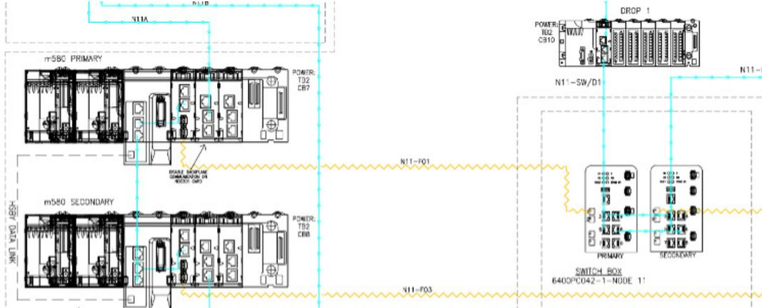
Figure 1. Hot standby PLC architecture
